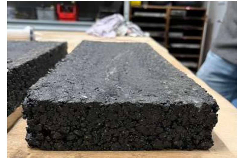
ASPHALT FOLDER IN STANDARD SB250 v.4.1 (WITH ASPHALTIC MIXTURE CONDITIONER)
